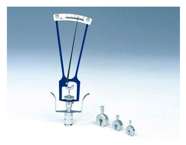
The product is used to measure the intraocular pressure (IOP) by measuring the depth produced on the surface of the cornea by a load of a known weight.
